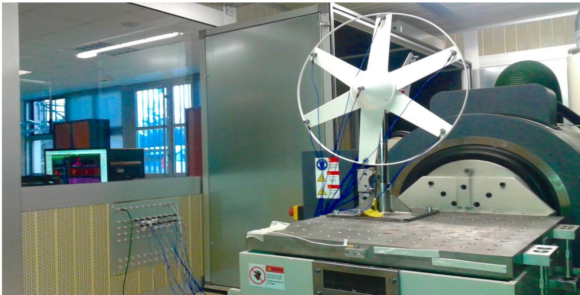
Fig. 3 Experimental Vibration-test platform of ECAM-EPMI Treviso-laboratory carrying the Rutland 504 wind turbine and the test instrumentations
