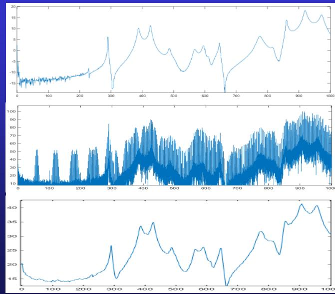
FRF measured using force and response
