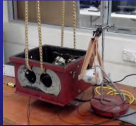
Gearbox casing excited by a shaker signal with 22 orders of a “shaft speed” with a mean of 76 Hz, but varying around this by  $\pm 15\%$ , with a modulating frequency of 2 Hz (0.5s period). This was to simulate a varying speed gearbox. The intention was to carry out OMA on the casing from the response signals only, but the shaker force was measured so as to compare with EMA
