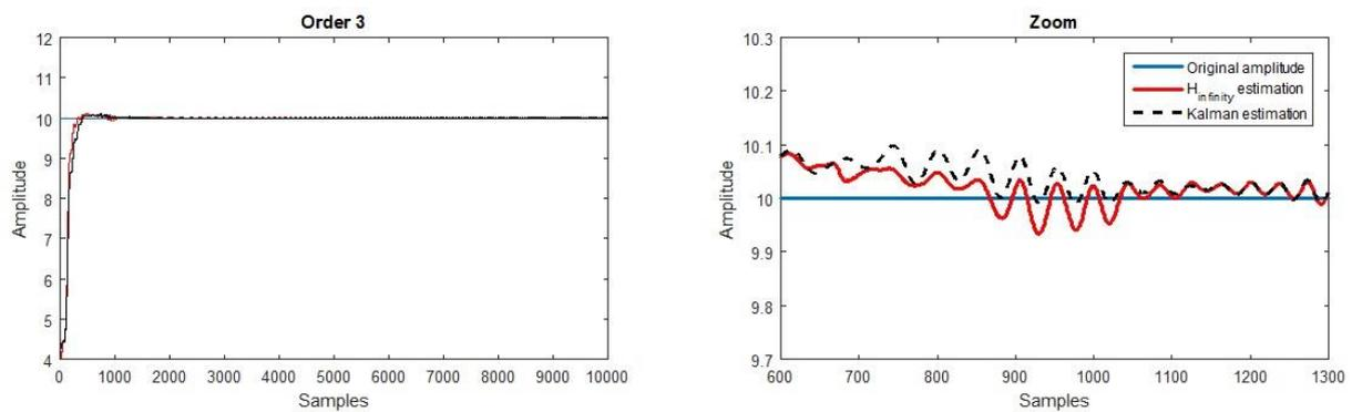
Fig. 6. Amplitude of order 3 estimated using the  $H_{\infty}$  and the Kalman estimator
