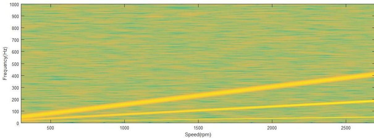
Fig. 2. Illustration of rpm-frequency spectrum
