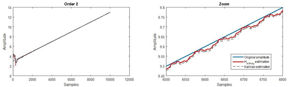
Fig. 5. Amplitude of order 2 estimated using the  $H_{\infty}$  and the Kalman estimator
