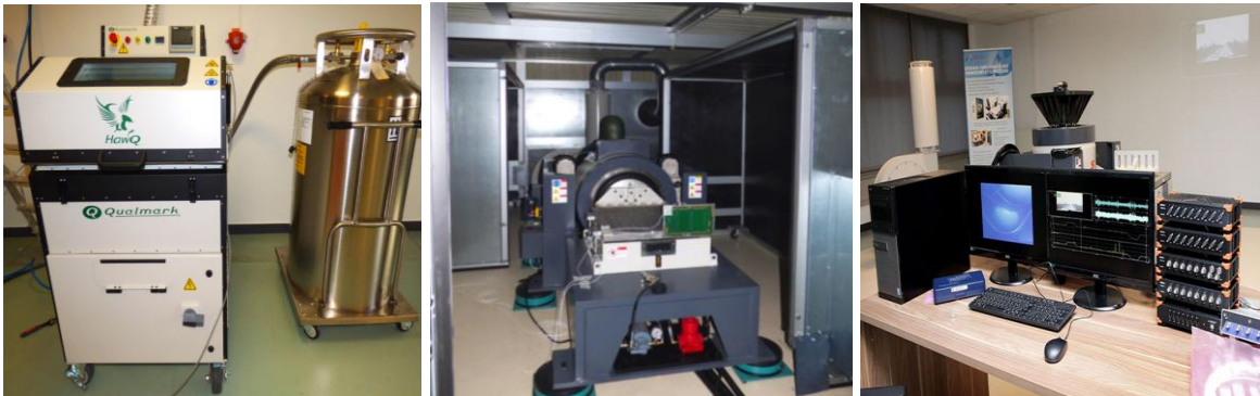
Fig. 3. Components of the vibration analysis platform TREVISE: the machine for vibro-climatic tests, TREVISE vibrator and the data acquisition package.
