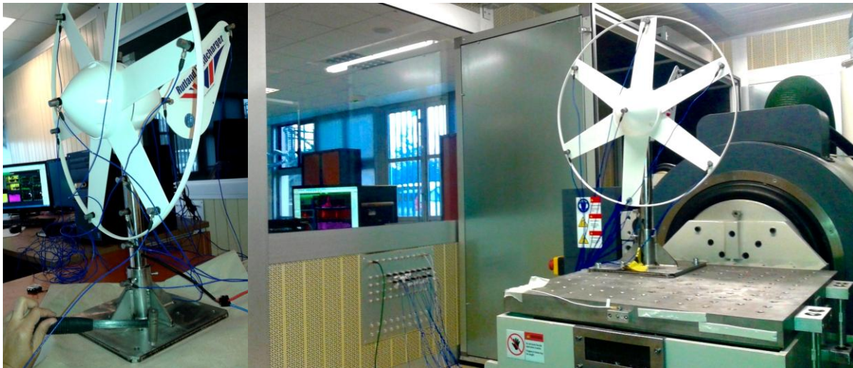
Fig. 5. TREVICE platform with the small-scale wind turbine and the test instrumentations: the calibrated hammer test (left) and TREVICE vibrator test (right).
