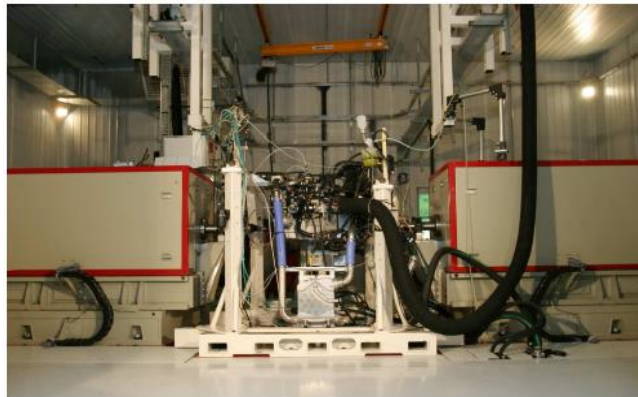
Fig. 14. In-situ measurement on the test bench with driveshaft suspension system.
